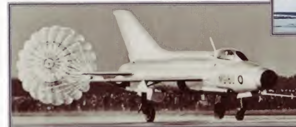
▼ Stopping aid Despite being a very light aircraft, the MiG-21 still required a braking parachute to slow it down upon landing.
